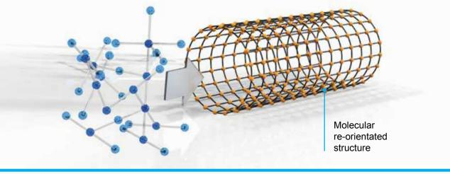
All of **A-SAFE's** products are made from **Memaplex**<sup>™</sup>, a robust and flexible polyolefin blend of materials with rubber additives. It's a three layered material that's exclusively manufactured by **A-SAFE**. Three combined zones, which has a make-up of eight blended polyolefin and rubber materials.
